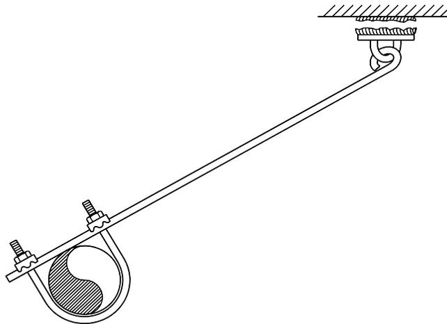
*Figure 3.4.5-2 Undersize Weld May Shear*
