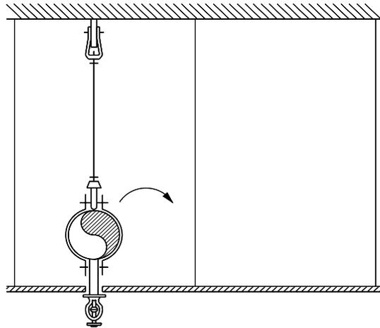
*Figure 3.4.3-2 Sprinkler Pipe Sways and Impacts Suspended Ceiling*
