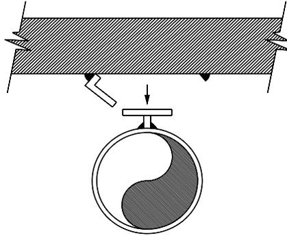
*Figure 3.4.5-3 Undersize Angle Weld, May Shear*
