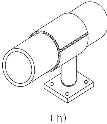
*Figure 8.2-2 Steel Pipe Anchor*
