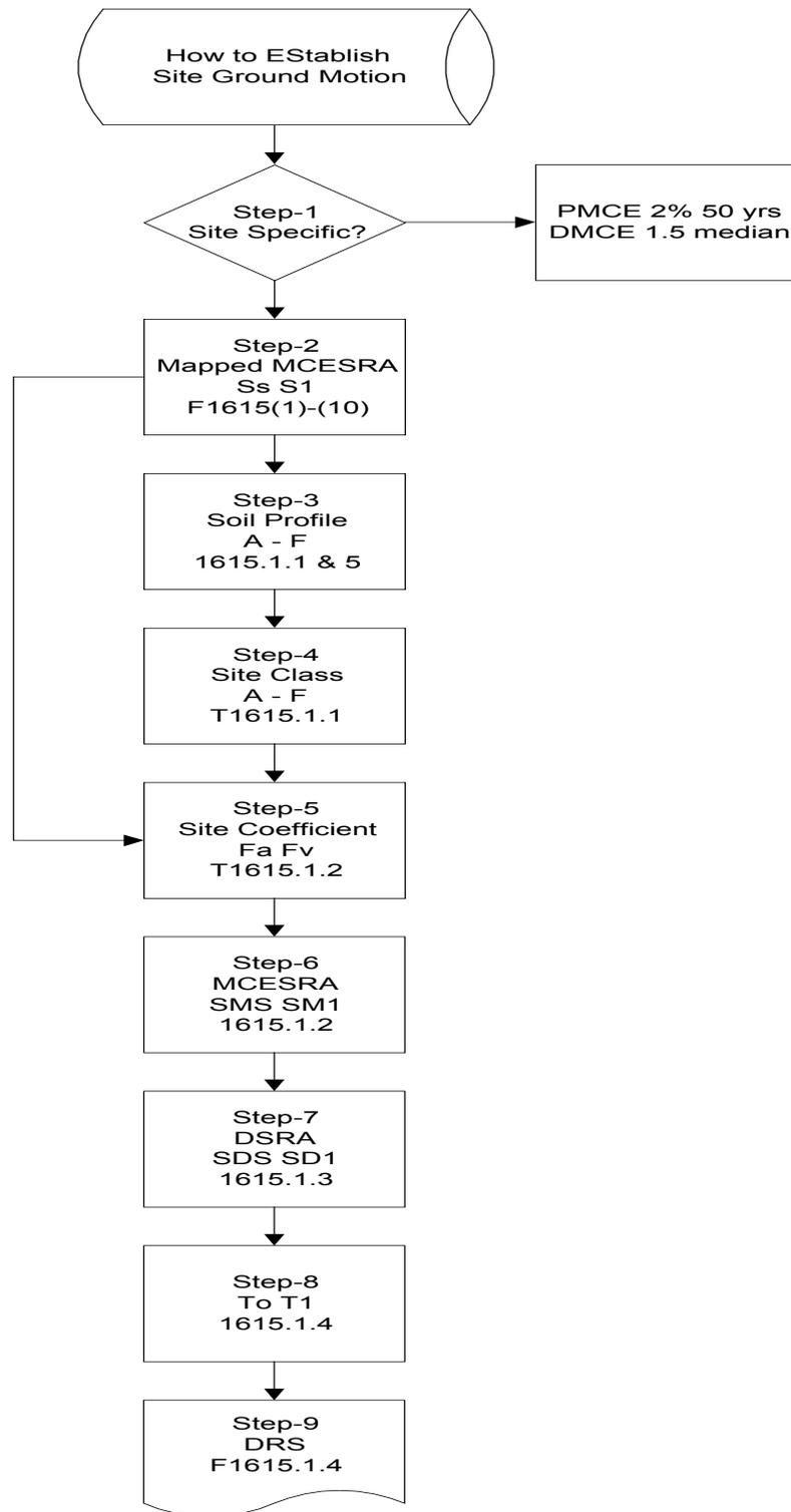
Figure 4.3.1-1 Determination of Site Ground Motion per IBC
