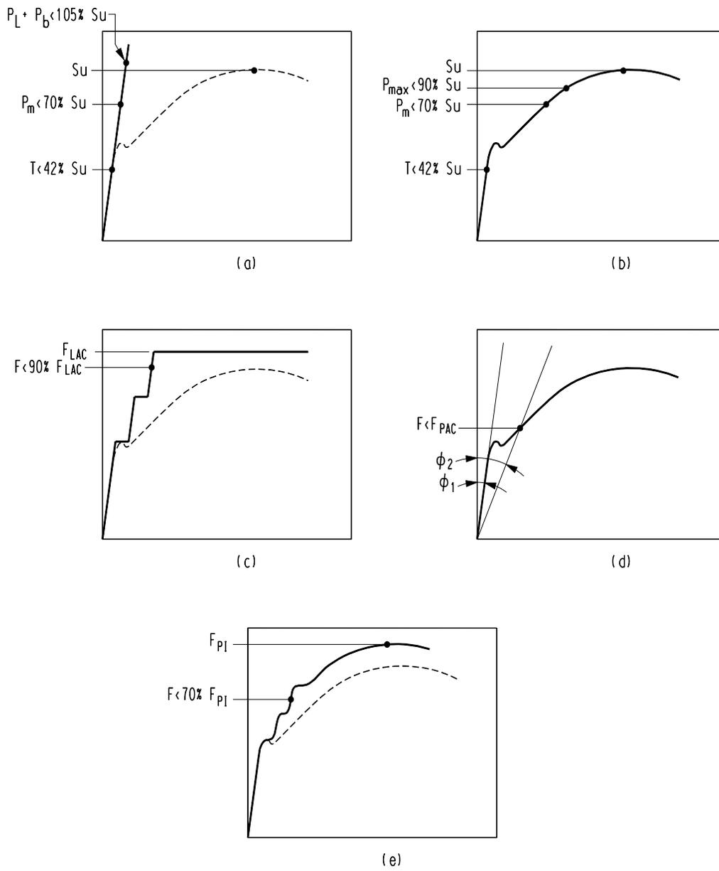
Figure 7.3-1 Analysis Techniques for Faulted Loads
