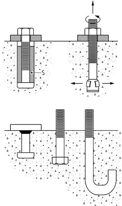
*Figure 8.3.1-1 Shell Anchor (top right), Non-Shell Anchor (top left), Cast-in-Place (bottom)*
