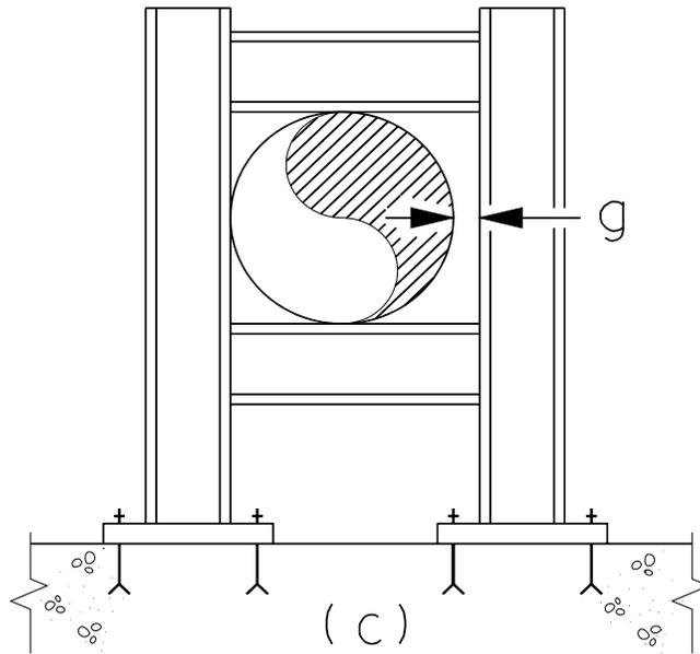
*Figure 8.2-1 Rigid Frame as a Lateral Seismic Support*
