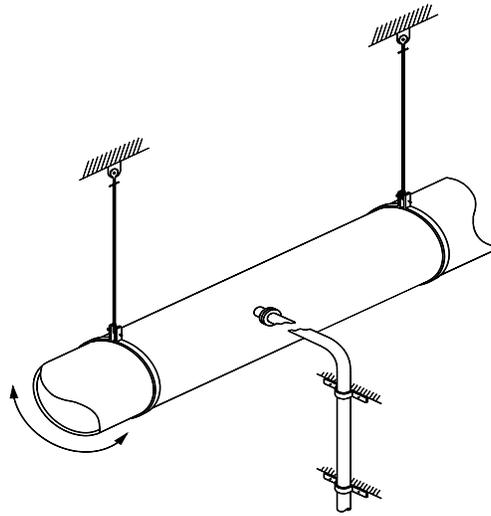
*Figure 3.4.4-1 Suspended Header and Stiff Branch*
