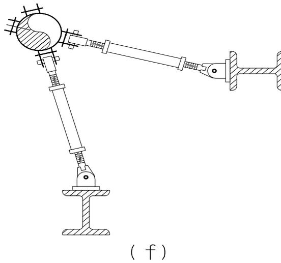
*Figure 8.1-2 Rigid Struts Sway Braces*
