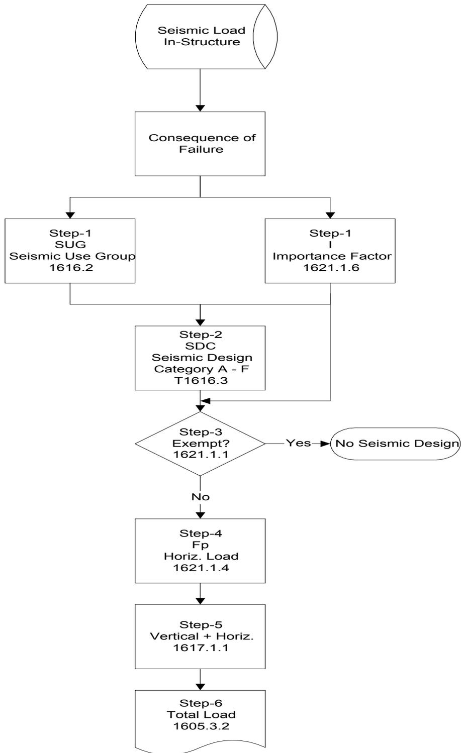
Figure 4.3.2-1 Determination of Seismic Load per IBC
