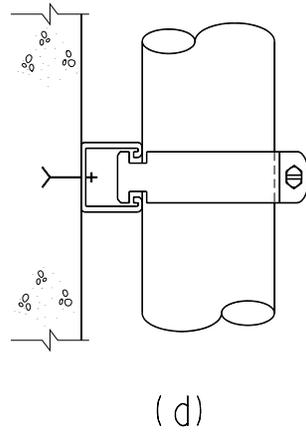
*Figure 8.1-3 Wall Mounted Strut with Pipe Clamp*
