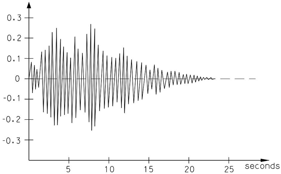
Figure 4.1.1-1 Illustration of a Seismic Time History Acceleration
