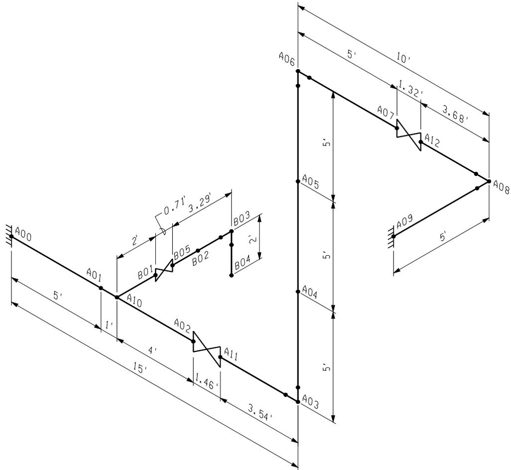
Figure C-3 Isometric of Example 1 Piping System
